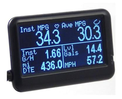
The UltraGauge MX has the ability to access non-standard, manufacturer specific gauges such as the transmission oil temperature.
